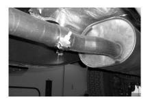
TO REMOVE YOUR STOCK EXHAUST, REMOVE IT FROM THE CLAMP LOCATED JUST IN FRONT OF THE MUFFLER. DO NOT DISCARD STOCK CLAMP, YOU WILL RE-USE IT. REMOVE HANGERS FROM RUBBER GROMMETS BY PULLING EXHAUST TOWARDS THE REAR OF THE VEHICLE, USE WD-40 TO AID IN REMOVAL, LEAVE GROMMETS IN PLACE.
