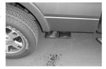
INSTALL STAINLESS TIPS, CLAMP DOWN. TO CLEAN YOUR STAINLESS TIPS USE ANY STAINLESS CLEANER OR A SCOTCH BRITE PAD. NOW GO AND TIGHTEN ALL CLAMPS, NUTS AND BOLTS. START FROM THE FRONT AND WORK BACK.
